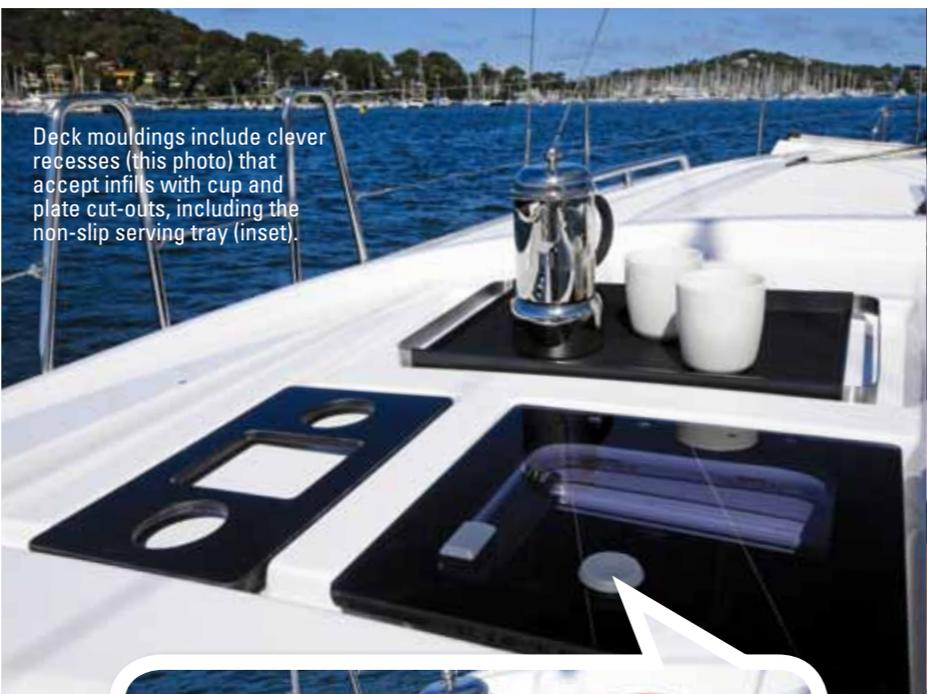
Deck mouldings include clever recesses (this photo) that accept infills with cup and plate cut-outs, including the non-slip serving tray (inset).
